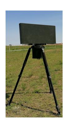
AUR-80 is a multi-functional battlefield surveillance radar that can be quickly deployed. It adopts the X-band continuous wave system. It mainly searches and detects ground active targets, and also takes into account the reconnaissance and detection of low-altitude targets. It is mainly used for alerting and reconnaissance in the combat area. It can automatically detect and locate moving ground personnel (single and crowd), vehicles, drones, small aircraft and other targets
