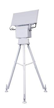
The AUR-30 is a rapidly deployable multifunctional surveillance radar. It adopts the Ku-band continuous wave phased array system, which can detect flying targets and provide various parameter information of the target, such as distance, azimuth, altitude and speed. It can track the target after it finds it, and display the target track on the terminal interface in real time, and send it to the weapon system to provide target indication.
