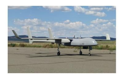
Size: wingspan: 8.00m, Length: 6.08m, Altitude
