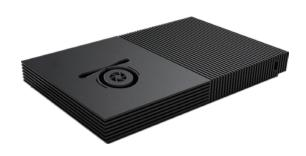
QT-14 gas detector is mainly used to detect the temperature, humidity, COz, PM2.5, PM10, PM10 and H2S, NO2, SO2 CH:, 0: and other related gas concentration data in the environment. It can view the detection data in real time, view the historical data, view the flight path on the map, and compare the data at different times in the same place.
