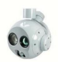
Q-30'I IVI IS a protessional nign precise three-axis stability augmentation zoom camera gimbal for drone.lt adopts high-precise encoder FOC control scheme, 30x optical zoom,1500m laser ranging, 640 x 480 thermal imaging pixels, and supports tracking. it has the characteristics of high stability, small size, light weight and low power consumption.
