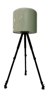
The navigation decoy device conducts navigation deception to the UAV by emitting simulated satellite navigation signals, so that the UAV will have the illusion of speed out of control, so as to drive the flying UAV away and return, stay away from the defensive area, prevent it from flying into sensitive areas, control The purpose of the black flying drone.
