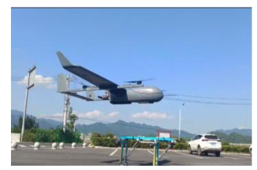
Size: wingspan: 6.12m, Aircraft commander: 3.57m
